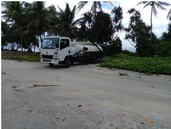
Figure 4: PWD/WSD septage pump out truck discharging its load of raw septage
